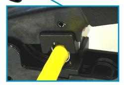
Allows you to clamp the cable screen on the cable insulation
