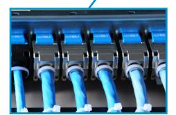
Metal construction ensuring galvanized connection with module shielding
