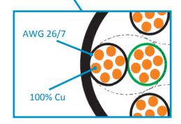
Prepared on cable with 26/7 AWG wire diameter, 100% CU
