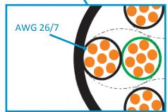
Prepared on cable with 26/7 AWG wire diameter
