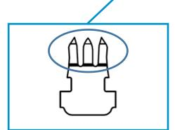
The triple pin blades provides higher electrical conductivity
