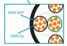
Prepared on cable with 24/7 AWG wire diameter, 100% CU
