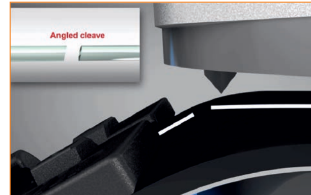
15. Pick down side with cable (now you are creating angle on end of fiber)
