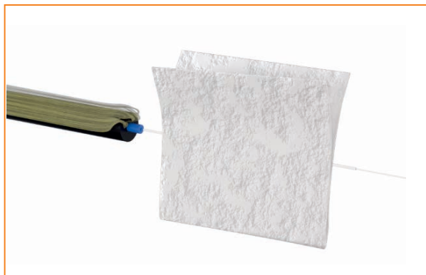
7. Clean the part of removed by the us of an alcohol wetted swab
