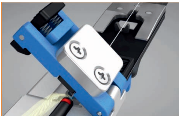
16. Open jig and demount cable
