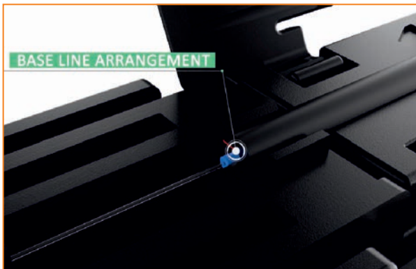
22. Set cable to the base line
